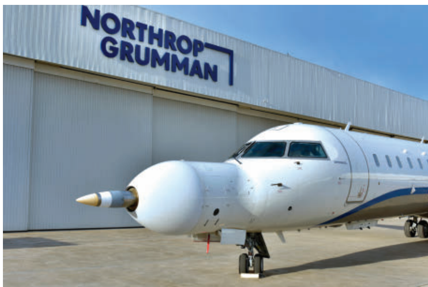
Northrop Grumman has employed a CRJ-700 testbed to conduct flight trials of a multimode sensor suite and mission computer intended to meet SiAW requirements. NORTHROP GRUMMAN
