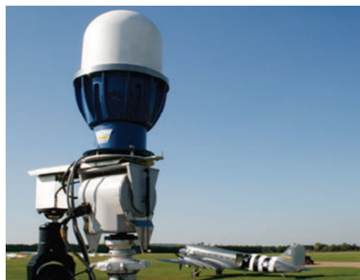
6 EHF Radar installation
