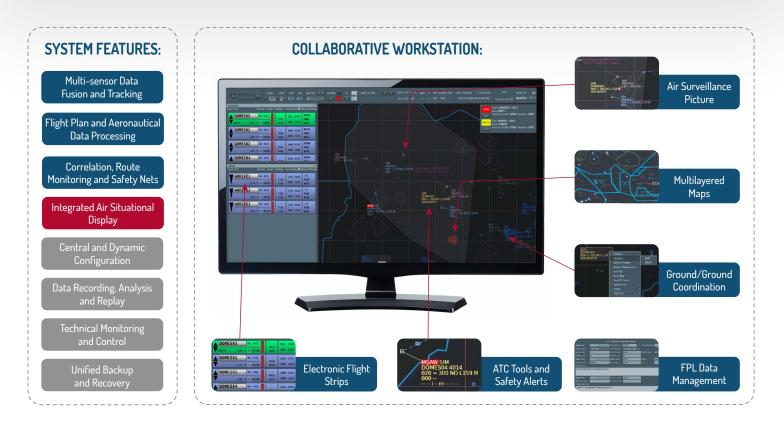
ERIS-ATM is suited for En-route and Approach application both at civil and military ATC centres. The situational picture is based on surveillance technology-oriented data fusion and tracking approach with continuous data integrity and quality check. In combination with available planning and auxiliary information and safety nets, ERIS-ATM supports the safety and efficiency of air traffic.
